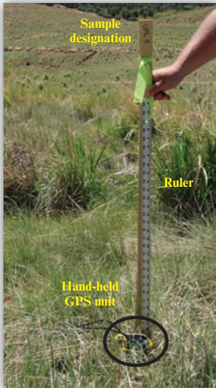
a. Vegetation height and GPS location measurement near Monticello, UT.
