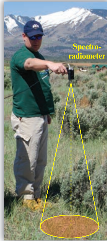
b. Spectral reflectance measurement of grassland near Monticello, UT.
