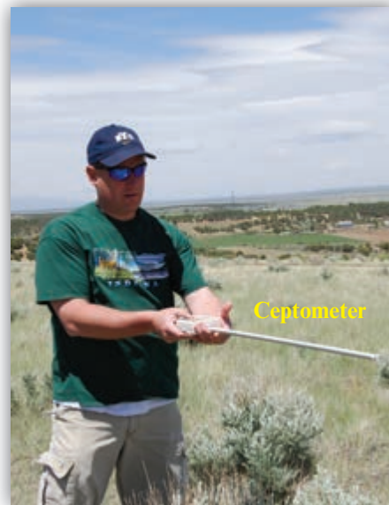
d. Above-canopy calibration of a ceptometer used to measure leaf-area-index (LAI) near Monticello, UT.
